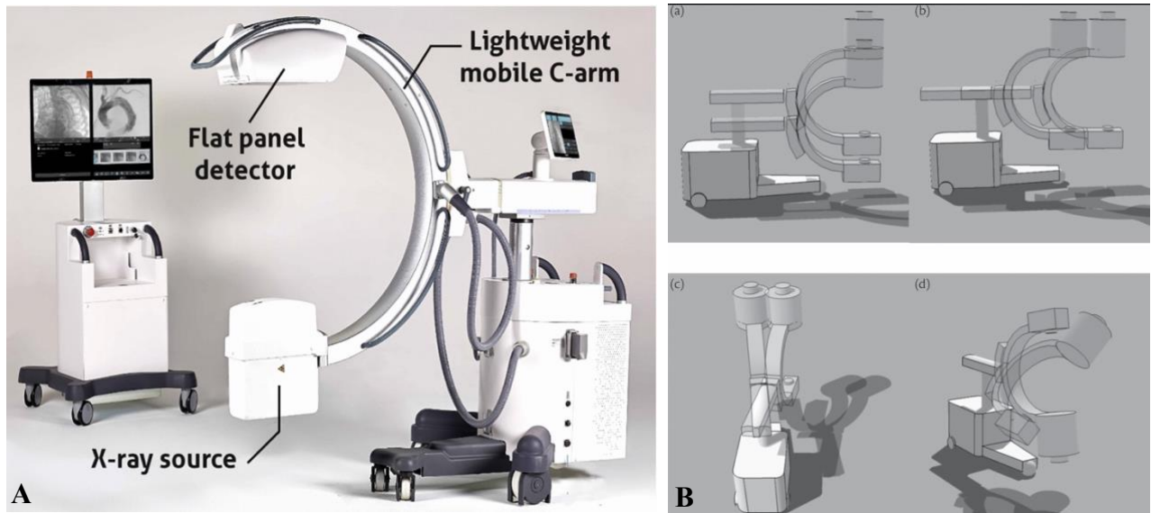
Figure 9. A: Labelled image of a commonly used mobile C-Arm system (ARCO FP by ATS) [19]. B: Common C-arm movements. (a) Vertical movement of the C-arm. (b) Horizontal movement of the C-arm. (c) Right/Left angulation. (d) Craniocaudal angulation [18].
